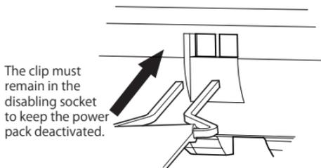
The clip must remain in the disabling socket to keep the power pack deactivated.
